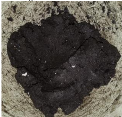
Fig. 1. The mixture of obsolete sludge and peat
