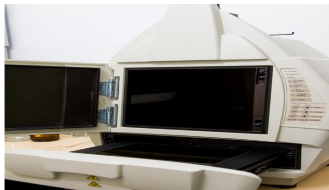
Video system for taking photographing of electrophorogramme of PCR products (BioRad, USA)
